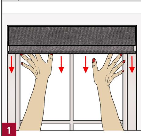
Gently **REMOVE endcap** from **non-control (idle)** side of cassette headrail.
