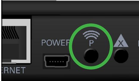
**2** **NOTE:** The solid green light on the Repeater will go out, indicating that it has been paired to the Hub.
